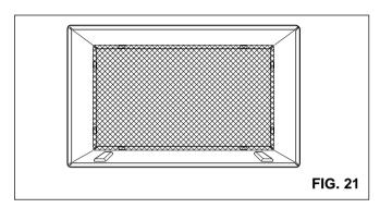
2 Fasten the 4 washer screws to secure the grille to the wall sleeve. If you need plastic nuts to mount plastic grille to the inside of the wall sleeve, there are plastic nuts in the installation kit. The nuts are installed from the inside of the sleeve and are pressed into the square holes of the rear flanges.
